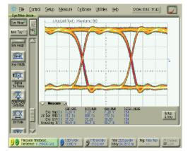
$\begin{array}{l} \textbf{Output response} \\ \textbf{Eye amplitude} = 7.3 \ \textbf{V}_{pp'} \ \textbf{Rise time} = 12.4 \ \textbf{ps} \\ \textbf{Jitter RMS} = 712 \ \textbf{fs}, \ \textbf{SNR} = 37.5 \end{array}$
