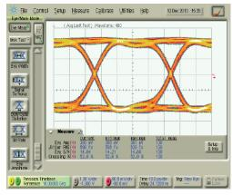
Input signal Eye amplitude = 0.5 V<sub>pp</sub>, Rise time = 12.4 ps Jitter RMS = 598 fs, SNR = 14.6
