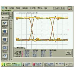
Input signal Eye amplitude = 0.5  $V_{pp'}$  Rise time = 9 ps Jitter RMS = 309 fs, SNR = 41
